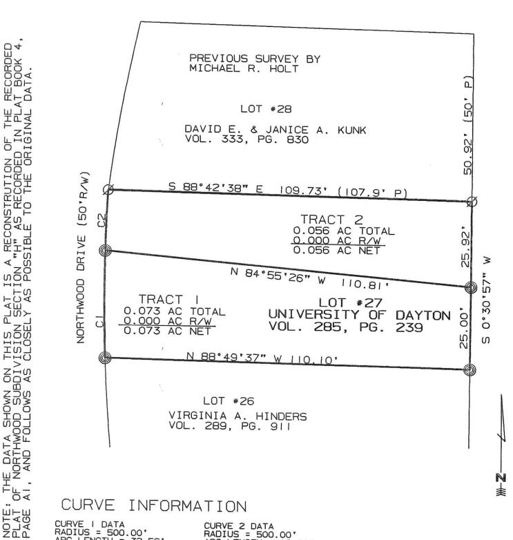
CURVE | DATA RADIUS = 500.00' ARC LENGTH = 32.56' DELTA = 3°43'50" CHORD = N 00°07'58" W 32.55' CURVE 2 DATA RADIUS = 500.00' ARC LENGTH = 18.61' DELTA = 2°07'56" CHORD = N 02°47'55" E 18.61'
